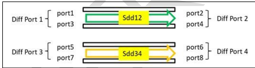
Figure 9-13 2 Differential Pair Port Map
