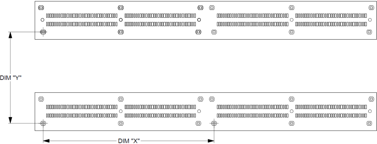
Figure B-3: Minimum Connector Spacing Requirements for 144P Connector
