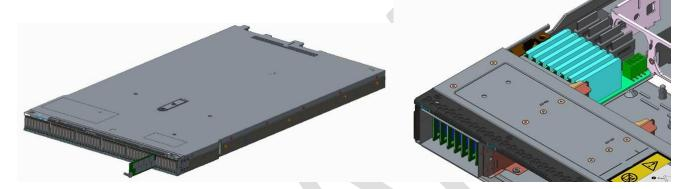
Figure 4-1. Example systems showing implementations of 1U short form factor.
