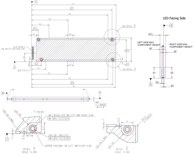
Figure 5-1. 5.9 mm Thick 1U Short Form Factor drawing
