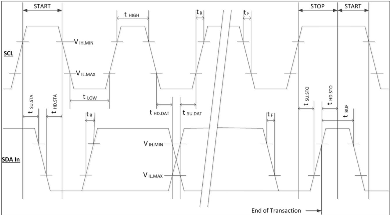
Figure 5-7 Timing Diagram
