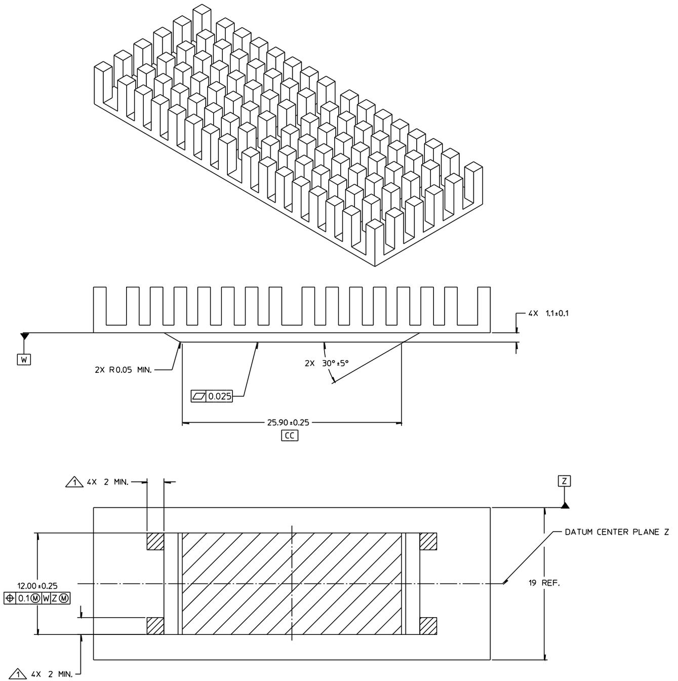
1. PLANE FOR FLATNESS AND HEIGHT MEASUREMENTS ESTABLISHED AT FOUR INDICATED AREAS
