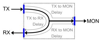
Figure 13-1 Calibration Loopback Module
