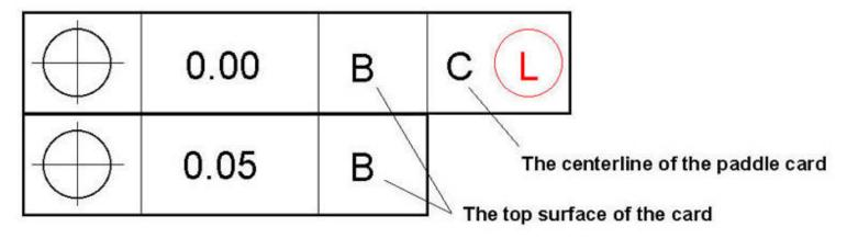
The 0.00 defines the positional tolerance of the paddle card pads to the centerline of the paddle card.
