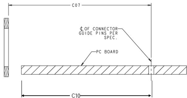
Side View Elastomeric EMI Gasket
