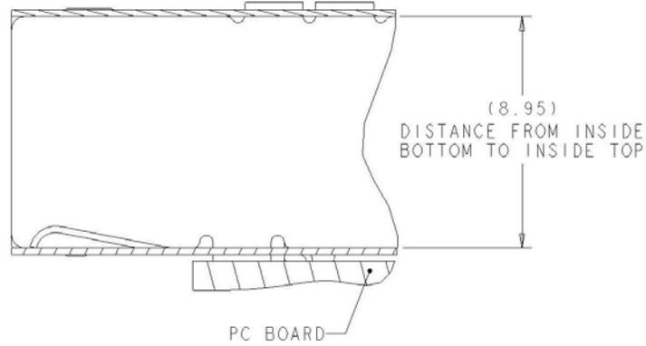
FIGURE 6-2 SECTION VIEW OF CAGE ASSEMBLY, INF-8074I
