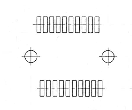
FIGURE 6-1 ILLUSTRATION FOR CONNECTOR PC BOARD LAYOUT, SFF-8083
