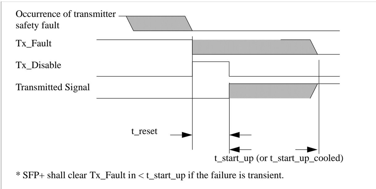
FIGURE 9 SUCCESSFUL RECOVERY FROM TRANSIENT SAFETY FAULT CONDITION
