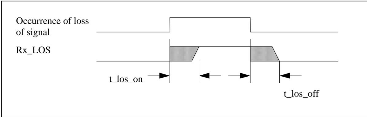
FIGURE 11 TIMING OF RX\_LOS DETECTION
