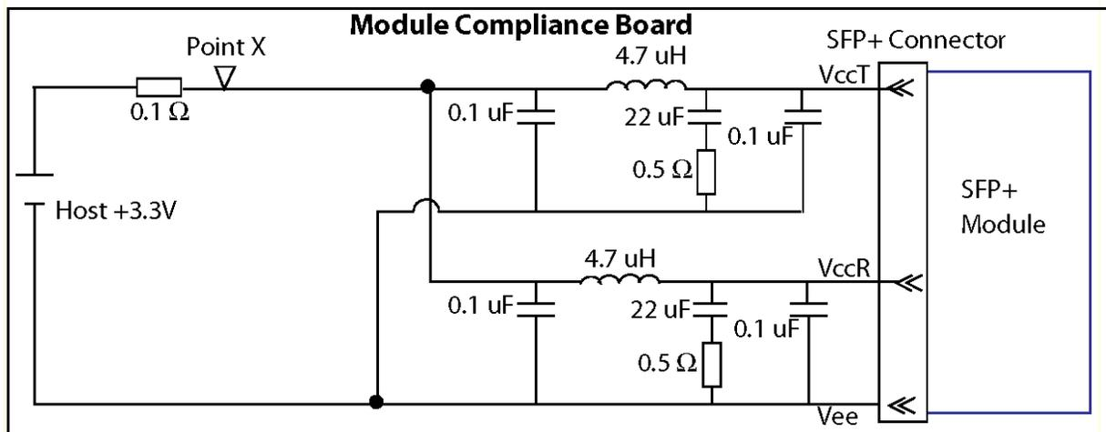
FIGURE 20 MODULE COMPLIANCE BOARD POWER SUPPLY FILTERS
