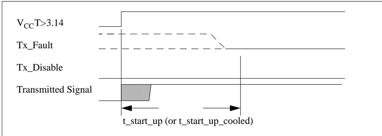
FIGURE 4 POWER ON INITIALIZATION OF MODULE, TX\_DISABLE NEGATED
