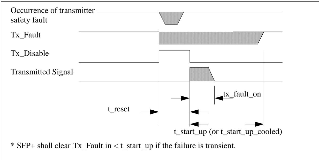
FIGURE 10 UNSUCCESSFUL RECOVERY FROM SAFETY FAULT CONDITION
