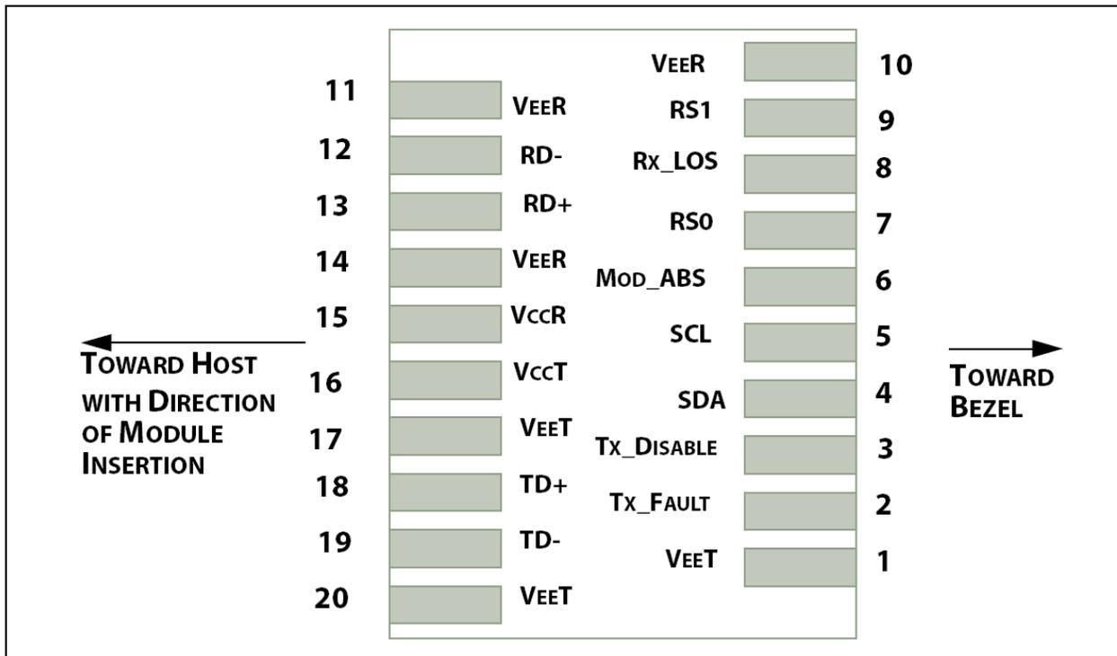
FIGURE 2 HOST PCB SFP+ PAD ASSIGNMENT TOP VIEW
