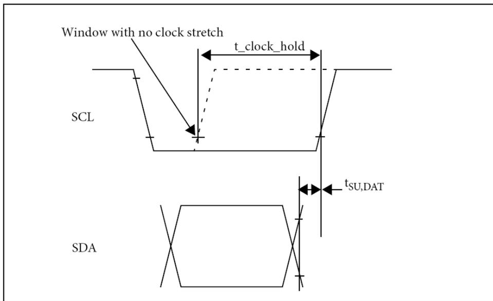
FIGURE 13 DETAIL OF CLOCK STRETCHING
