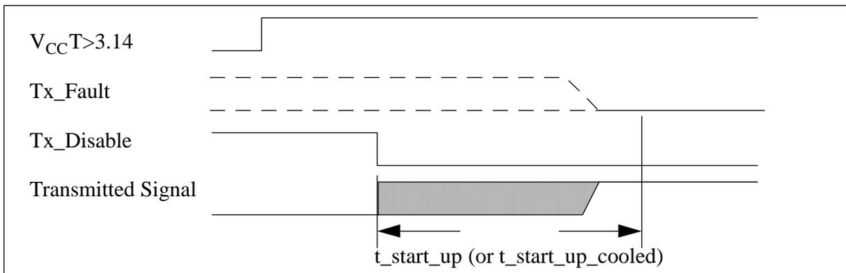
FIGURE 5 POWER ON INITIALIZATION OF MODULE, TX\_DISABLE ASSERTED
