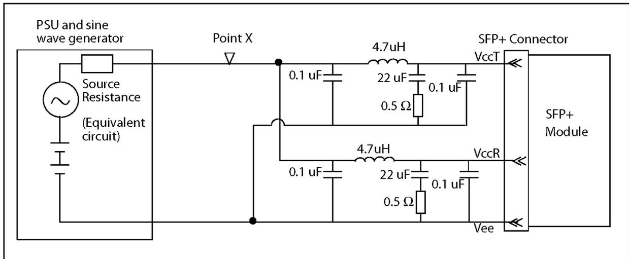
FIGURE 22 POWER SUPPLY NOISE TOLERANCE TEST SETUP
