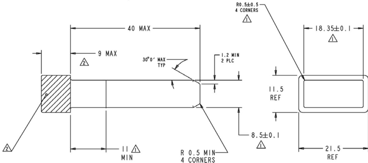
△ DIMENSIONS APPLY FOR INDICATED LENGTH. REMAINING LENGTH MUST NOT EXCEED MAXIMUM OF SPECIFIED DIMENSIONS.
