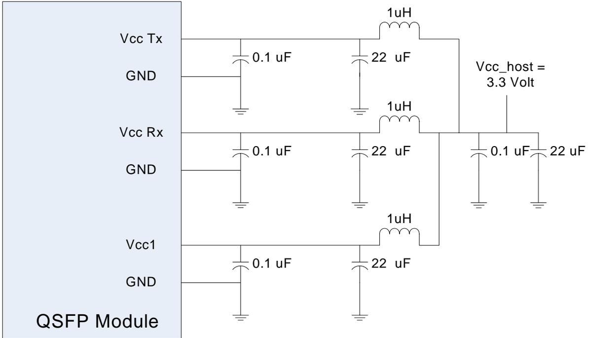
Any voltage drop across a filter network on the host is counted against the host DC set point accuracy specification. Inductors with DC Resistance of less than 0.1 Ohm should be used in order to maintain the required voltage at the Host Edge Card Connector.
