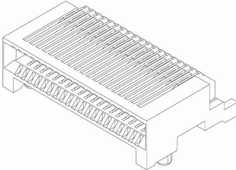
Figure 14 — QSFP Electrical Connector Specification
