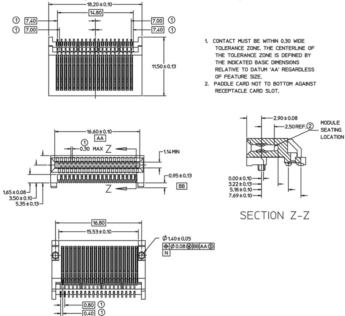
1. CONTACT MUST BE WITHIN 0.30 WIDE TOLERANCE ZONE. THE CENTERLINE OF THE TOLERANCE ZONE IS DEFINED BY THE INDICATED BASIC DIMENSIONS RELATIVE TO DATUM 'AA' REGARDLESS OF FEATURE SIZE.
